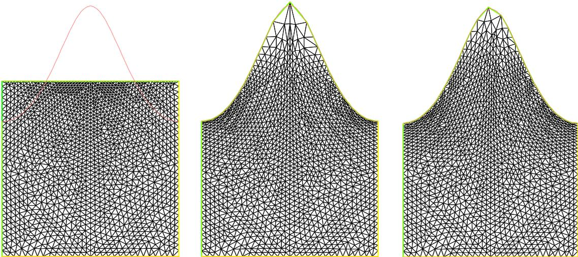
Figure 18: Left: reference mesh  $\mathcal{T}_{\text{ref}}$ ; Middle: deformed mesh  $\mathcal{T}_{\text{map}}$  using  $(\cdot, \cdot)_{\text{elas},F}$ ; Right: deformed mesh  $\mathcal{T}_{\text{map}}$  using  $(\cdot, \cdot)_{\text{elas},\kappa}$ .
